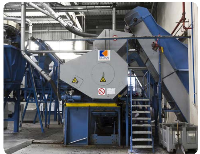
Rasper for processing of various materials (here shown in a tyre processing line).
