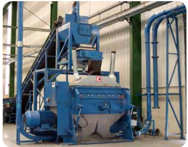
Eldan Heavy Granulator with closed inlet hopper processing WEEE.
