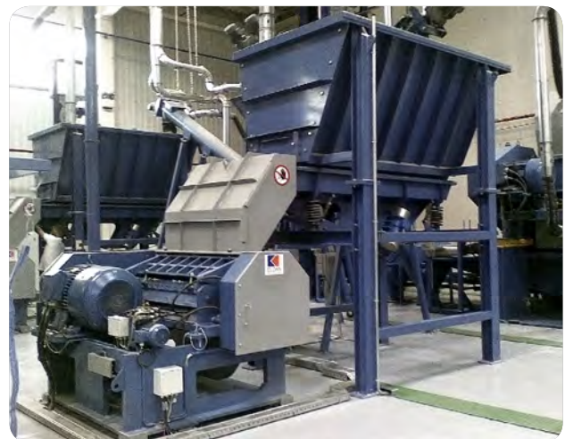
Fine Granulator as a part of a tyre recycling system. Feeding via a Silo (V4) to ensures optimum utilization of the capacity.
